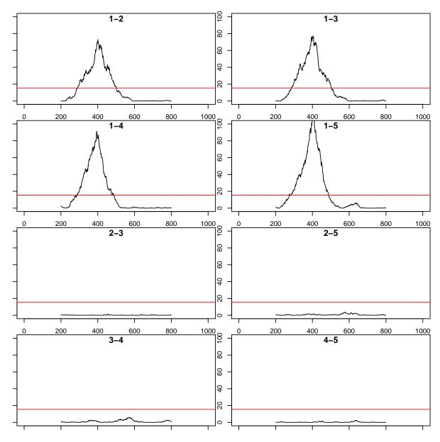
One can now clearly see that it is most likely that a change point occurred at time 400. This change point as well as its magnitude is also obtained through setting returnStat=FALSE in pairwiseSNHT. Furthermore, the corrected data can be accessed through *out2\$breaks* respectively *out2\$data*.
