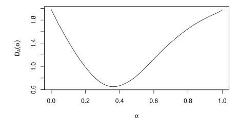
For knot.n = 1 we may find best knot.alpha using numerical optimization. It may be shown, see [5], that the distance function  $D_A(\alpha)$  is continuous, but in general the minimum is not necessarily unique.
